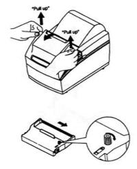
3). To use a new roll paper, unroll the paper and tear off the end of the paper correctly.
